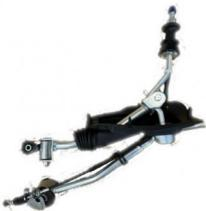
Quick gear shifting is achieved with an approximately 10% reduction in shift stroke.
