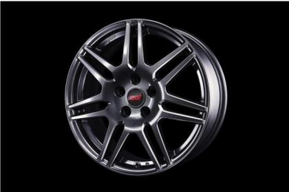
**WHEEL SET 18inch (GUNMETALLIC)**SG217SJ011 (B3110SJ011) GUNMETALLIC 18x7.0J/+48 PCD114.3
